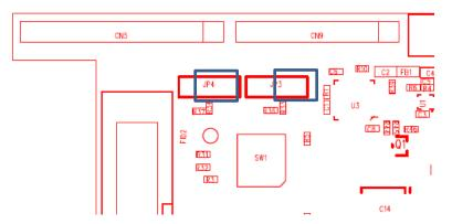
There are several options (selectable by 0-ohm resistive jumpers) for routing the UART signals to CN5/9 connectors – See previous section how to resistor jumper in these pins on the DU-EB!
