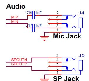
Note that the MIC feed **has been modified** from what is shown above. C16 now shunts the DHAN-J MIP pin to GND. Thus, the MIC input is now Line-In and fed by the right channel stereo connection as shown below:
