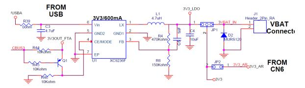
The 3.3V powering the DU-EB can be supplied from one of 3 sources:
