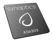
The AS6303 is a high-performance amplifier designed to drive capacitive loads of up to 10  $\mu\text{F}$ , such as piezo transducers. It integrates a 25 V boost converter, enabling Class H operation through an envelope-tracking architecture. The fine-grained booster, combined with advanced power flow management, minimizes current peaks in and out of the input supply for smooth system integration into portable devices.
