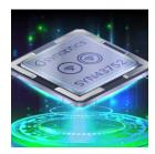
The Synaptics SYN43752 system on chip (SoC) combines a dual-band (2.4 GHz, 5 GHz) Wi-Fi 2×2 MAC/baseband/radio with Bluetooth 5.3 to reduce the space, cost, power, complexity, and time to market of IoT devices that demand robust and interoperable wireless connectivity.
