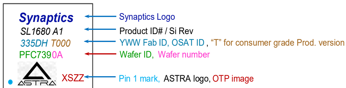
Figure 22. Package Marking and Pin 1 Location
