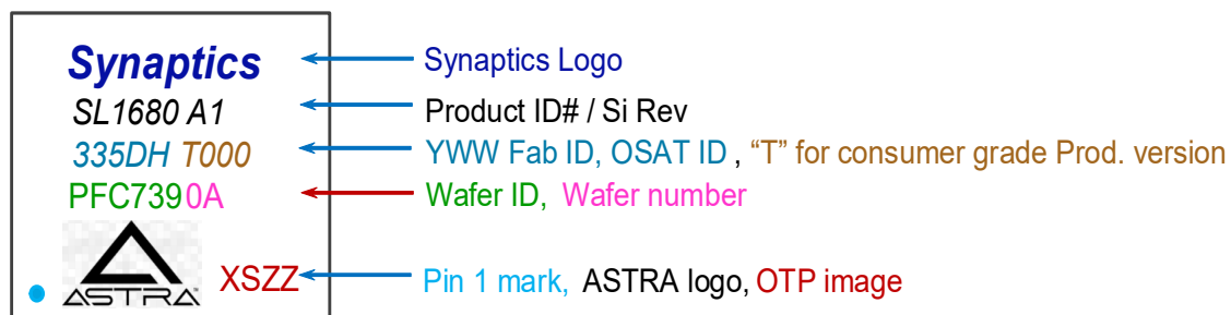
Figure 22. Package Marking and Pin 1 Location
