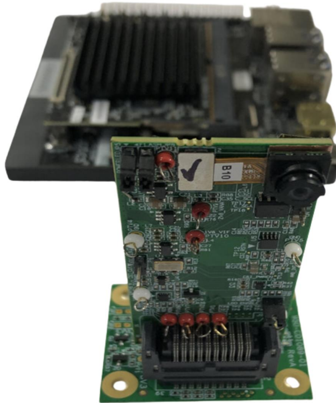
Figure 9. Connector connection with IMX258 module adapter
