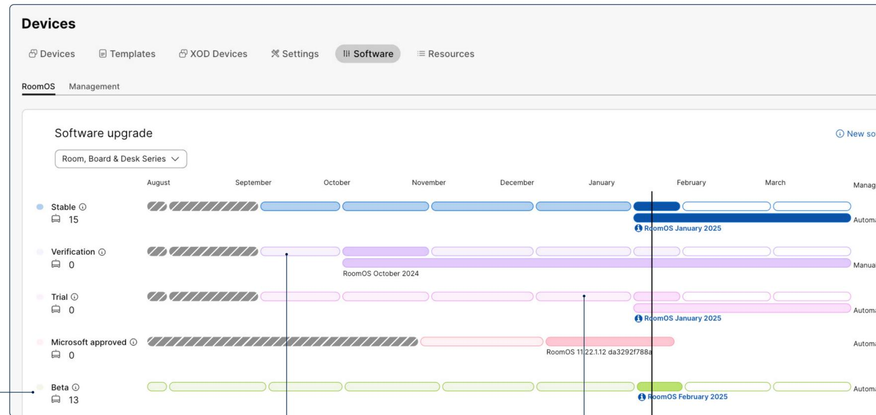
Use the Verification channel to test a newer release of production-ready software as your current release approaches its expiry date.
