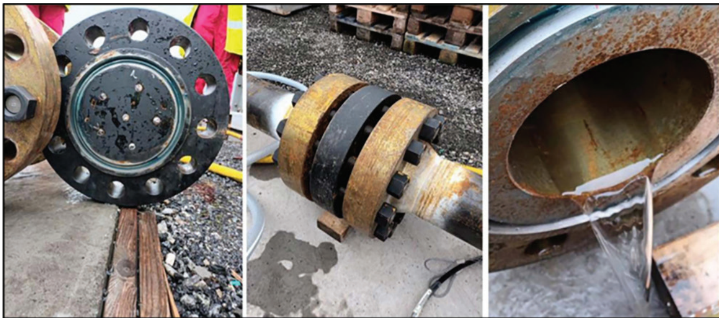
FIG. 2. Full-scale yard trial simulated subsea choke conditions and gel displacement behavior.
