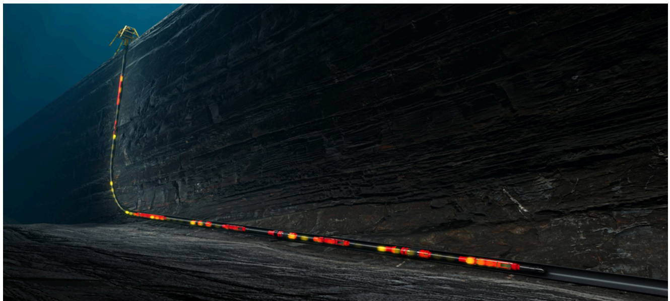
Fig. 2. An all-electric intelligent completion system allows precise zonal control and constant downhole diagnostics throughout the wellbore.
