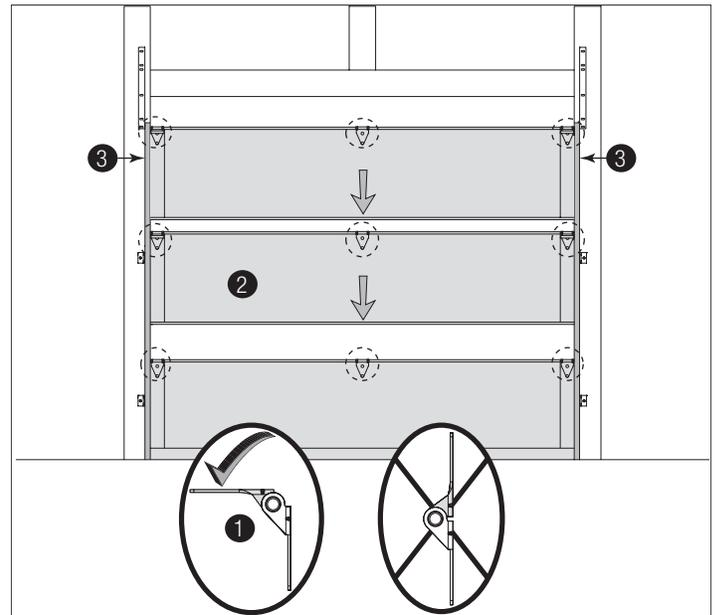
Figure 30, Stacking Sections
