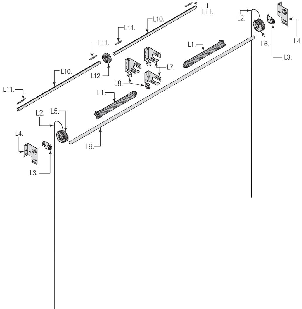
**Figure 7 - Counterbalance Components**
