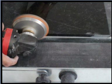
Rigid Backer Pad with Hat Trick Polishing Pads on the RTC grinder & Backdraft
