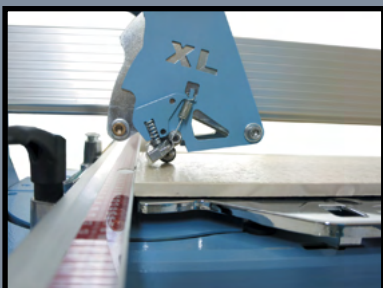
Spring loaded scoring wheel is ideal for all surfaces
