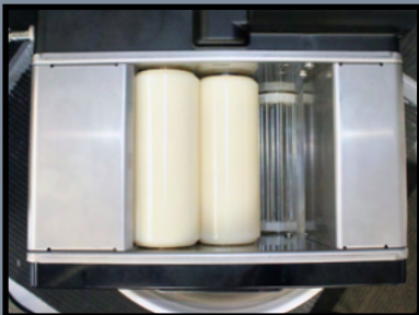
Spring loaded nylon rollers wring sponges virtually dry
