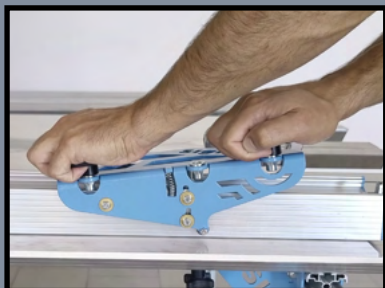
Two-handed scoring provides optimum pressure
