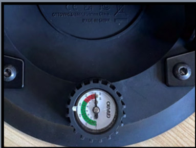
Pressure gauge visually ensures suction
