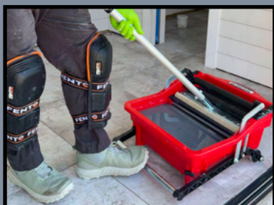
Pedal that controls double rollers for wringing sponge
