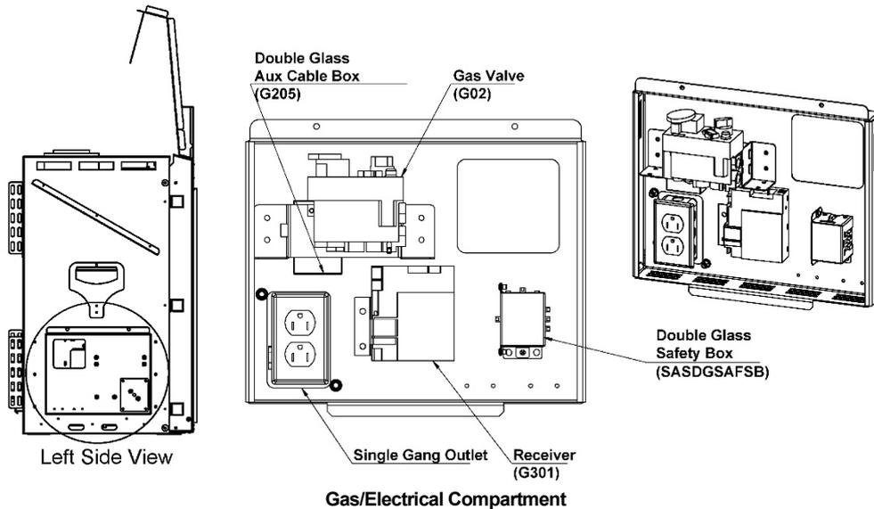
A gas shut-off valve and a 12" gas flex connector are provided with every fireplace. The location of the gas shut-off valve is dependent on local codes and requirements. Check with your authority having jurisdiction for more information.
