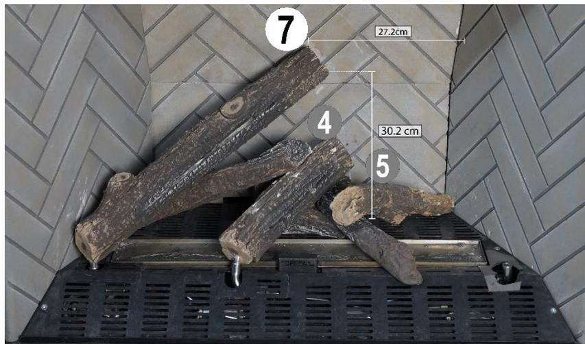
The base/tube for log #7 can be adjusted to fit the position shown in the picture above. (See “Log Base position Adjustment” section for details). Log #7 is 27.2cm from the right-side refractory and 30.2cm from the media tray.
