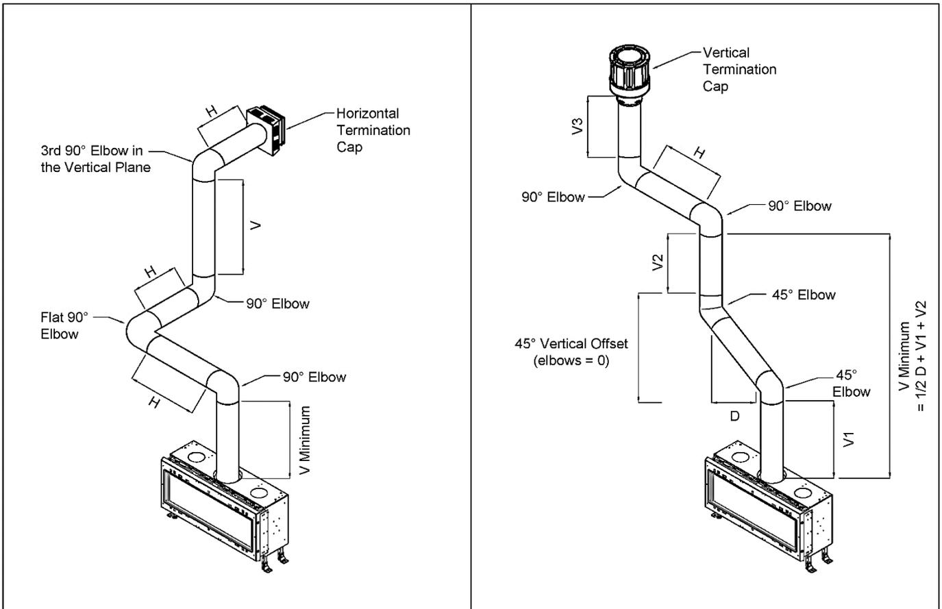
**! TERMINATION CAP NOTE:** Low Profile Termination Cap and Sconce Termination Cap can negatively impact flame appearance and are not recommended for use with the fireplace.
