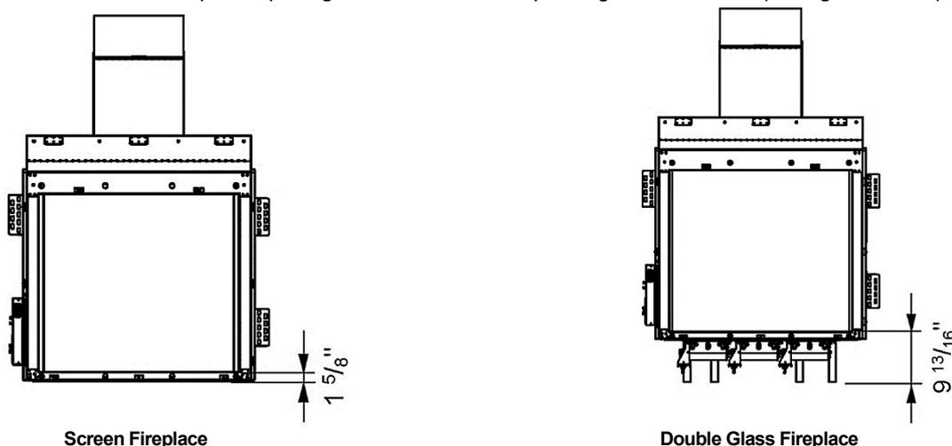
**Raised Platform Option:** To raise the fireplace higher than  $1\frac{5}{8}$ " for screen or  $9\frac{13}{16}$ " for double glass, build a platform for the fireplace to stand on. Platform must be stable and able to bear the full weight of the fireplace. A platform can be constructed out of wood, concrete, metal, or any other solid materials. Platform material is not required to be non-combustible.
