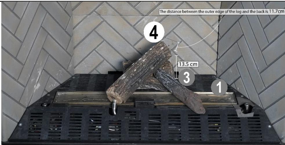
The base/tube for log #4 can be adjusted to fit the position shown in the picture above. (See "Log Base position Adjustment" section for details). The distance between the outer edge of the log and the back is 11.7 cm.
