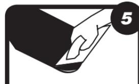
For Bonded Method only, apply a slurry bond coat.
