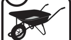
For hand mixing: Gradually add 3 to 4 U.S. qts. (2,84 to 3,79 L) of water or 3 to 3.5 U.S. qts. (2,84 to 3,31 L) of *Planicrete AC* to 55 lbs. (24,9 kg) of 4 to 1 while mixing with a mortar hoe.
