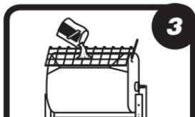
For machine mixing: Add 3 to 4 U.S. qts. (2,84 to 3,79 L) of water or 3 to 3.5 U.S. qts. (2,84 to 3,31 L) of *Planicrete AC*. Then add 55 lbs. (24,9 kg) of 4 to 1.
