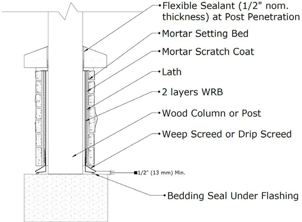
A minimum one half inch (13 mm) clearance should be maintained at all sides of the base. All column materials to be exterior grade. Do not extend flashing past edge of AMSV for safety reasons.
