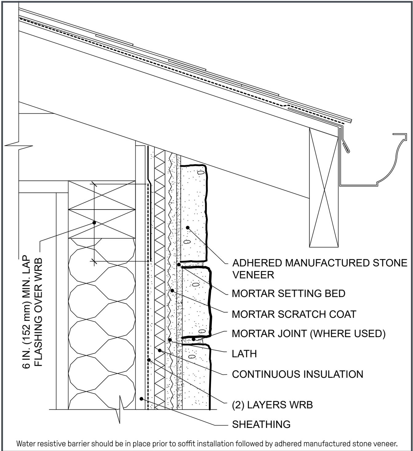
Water resistive barrier should be in place prior to soffit installation followed by adhered manufactured stone veneer.
