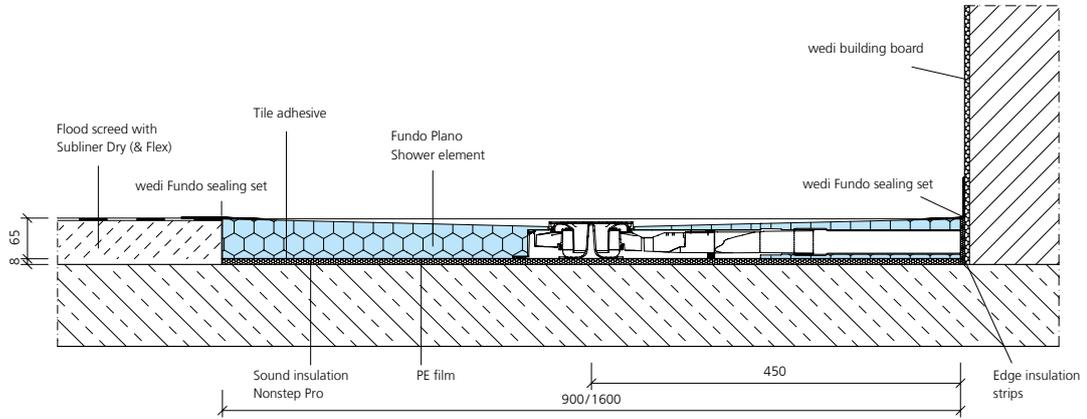
Fundo Plano, complete system A, connection on the long side
