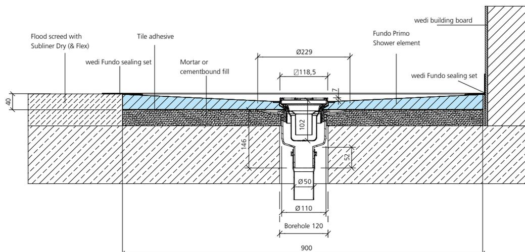
**i** The shower element Fundo Nautilo has a thickness of 50 mm.
