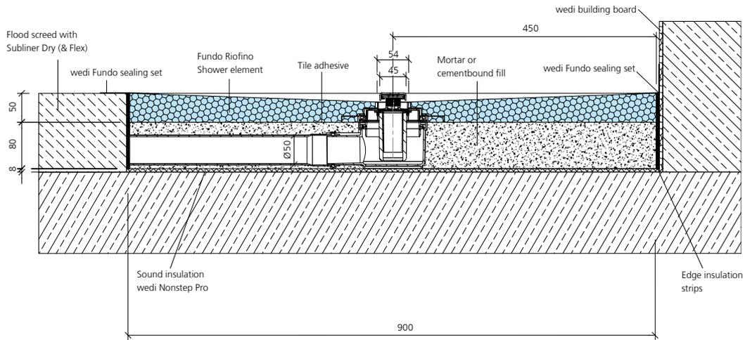
wedi Fundo channel drain Mini Max, DN 40, screed floor
