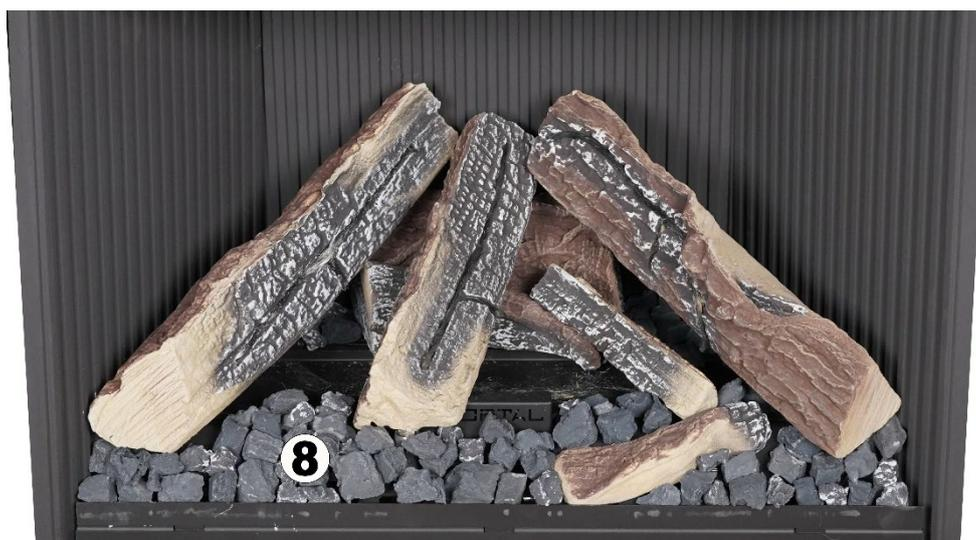
Add the charcoal pieces to the remainder of the burner. Do not cover burner holes. Maintain minimum 1-inch clearance around the pilot behind pilot hood.
