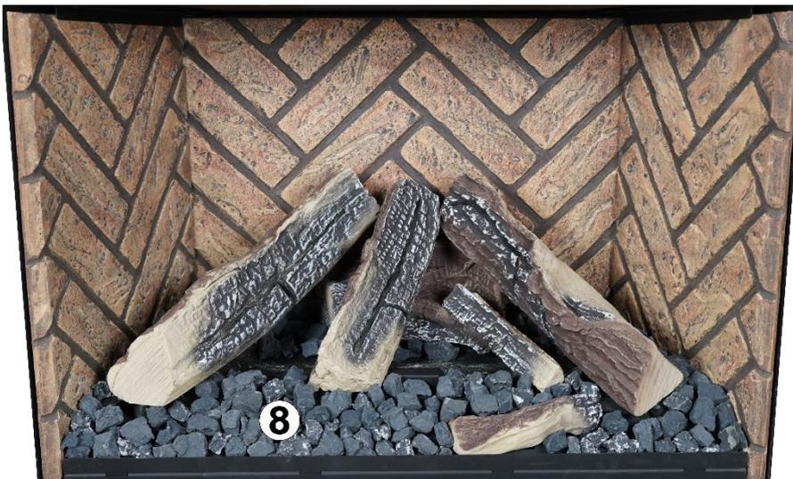
Add the charcoal pieces to the remainder of the burner. Do not cover burner holes. Maintain minimum 1-inch clearance around the pilot behind pilot hood.
