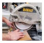
Make sure the wet saw has abundant water flow and cut slowly at 30 seconds or more per inch. Use a new piece of cardboard for cutting each tile. Keep saw table clean.
