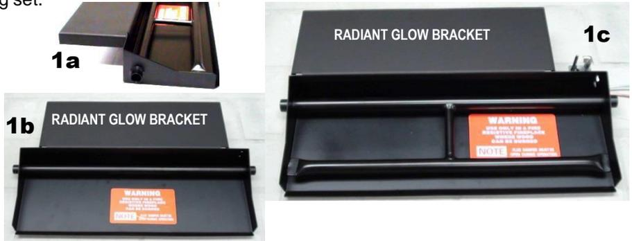
STEP 1: Figure 1a illustrates how the radiant glow bracket slides and rests on the back of the burner pan. For installation on burner pans without pilots center the bracket on the back of the burner pan as shown in figure 1b. For installation on burner pans with a pilot install the bracket on the back of the burner pan allowing 1" clearance around the pilot assembly as shown in figure 1c. The grate can then be pulled forward over the burner pan, as shown in figure 1e.
