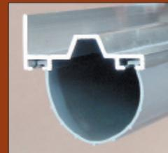
Reinforced Aluminum Bottom Extrusion Heavy duty grooved "U" type weather seal is set into an aluminum reinforced "L" angle, and bonded to the bottom section.
