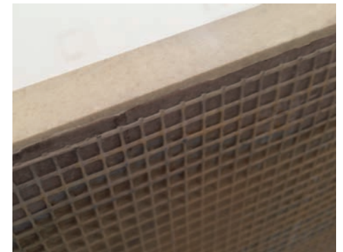
Backing with double fiberglass mesh.
