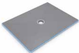
04 wedi Fundo Ligno Our newest Fundo model: Floor level 19 mm profile designed especially for suspended wood subfloors. Like all wedi shower bases it is pre sloped, and waterproof. Comes with 100 × 100 mm drain cover. Customisable on site.
