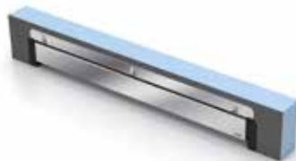
05 wedi Fundo Discreto Wall drain module for integration in seats or false walls. Installs over select Riolito neo linear drain models. Cover is tileable on one side and polished stainless steel on reverse side.
