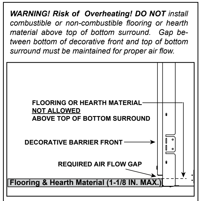
Figure 10.3 Required Air Flow Gap
