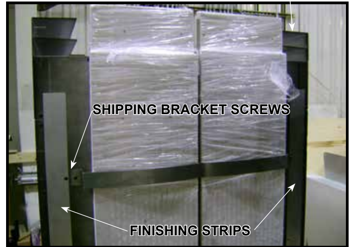
Figure 6.3 Shipping Brackets and Finishing Strip Locations.
