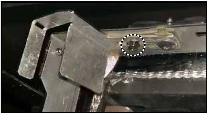
Figure 11.26 Shipping Location of Refractory Brackets
