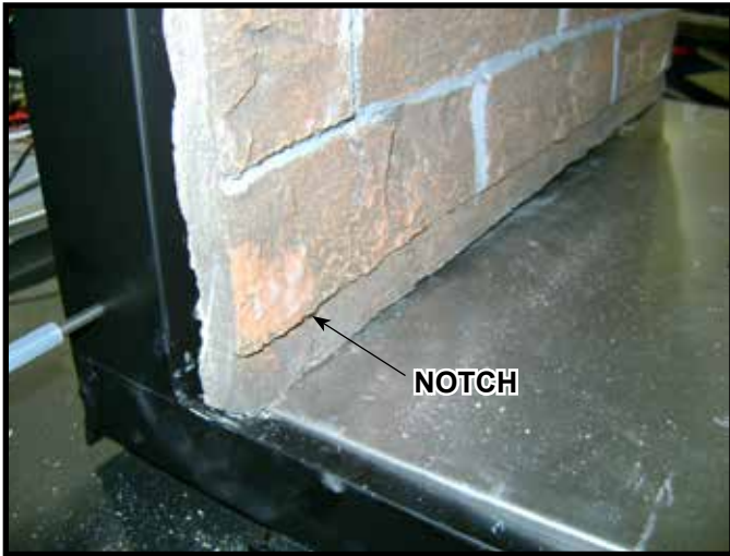
Figure 11.15 Notched End of Side Refractory
