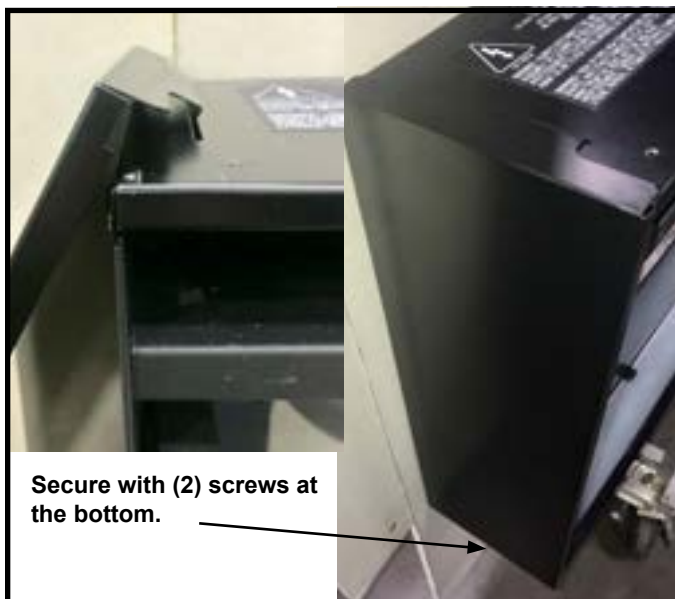
Figure 7 Installing Side Panels
