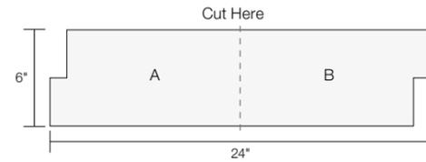
3. Corner panels should be cut into two pieces at desired lengths and finger joined around the outside corner as shown. One corner panel is needed to complete one linear foot of outside corner.
