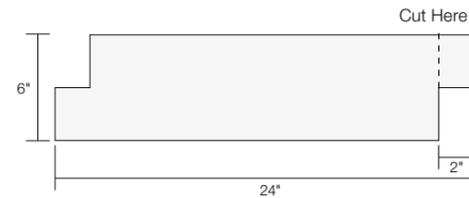
5. Alternate the size of the corner pieces to help stagger the joints. Do not stagger in a brick fashion, but randomly alter the size to conceal the joint patterns.
