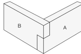
4. Continue installation by removing one staggered end of the plain ledger stone piece and place adjacent to the installed corner piece to continue row.
