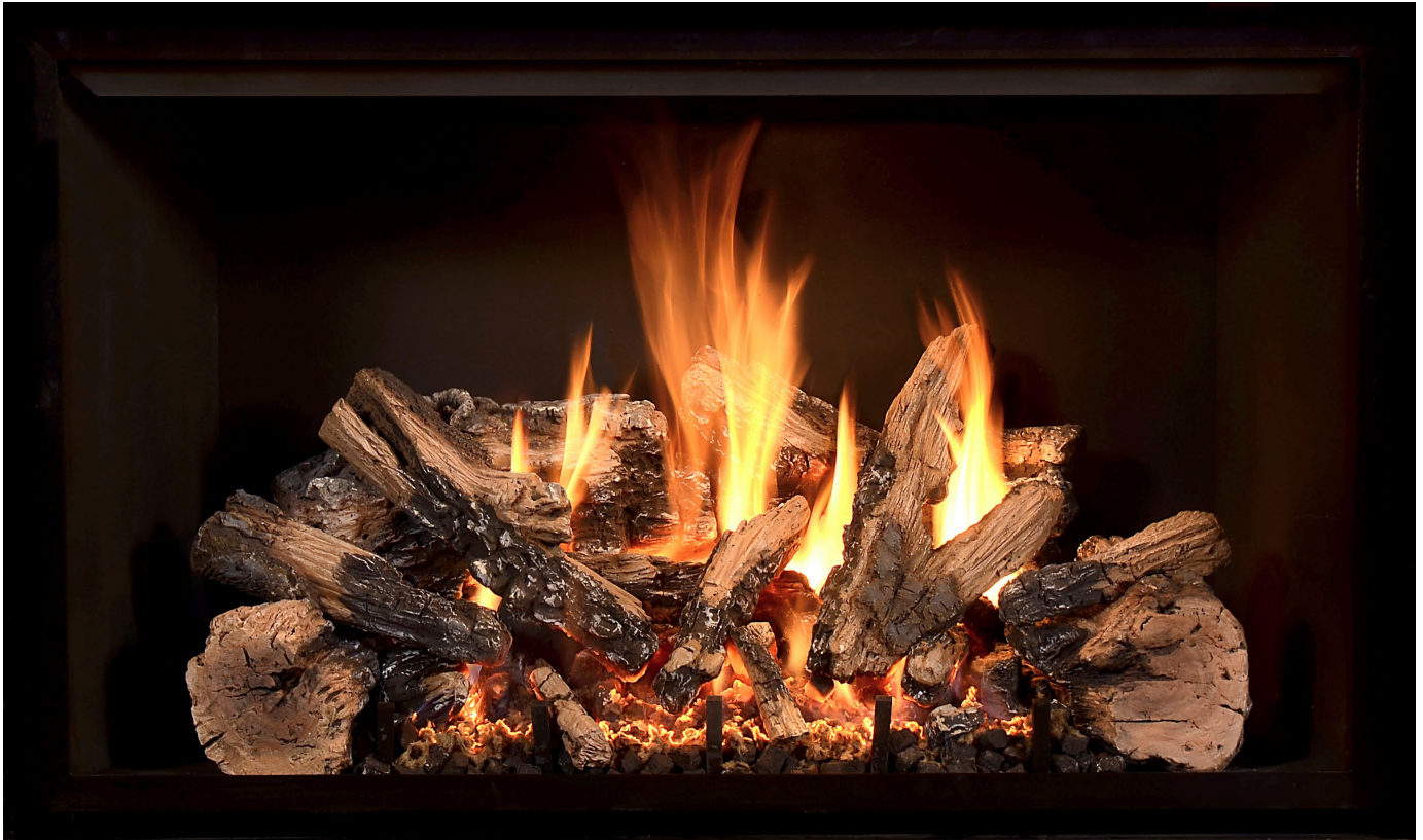
Figure 6-2 Burner Flame Heights: This image provides a visual reference for the burner flames burning at maximum height after the burners have been operating for 30 minutes or longer. A normal rear flame will be 1 to 2 inches above the rear log top edge. This, however, is dependent on the gas type, air shutter opening setting and vent system configuration. Actual flame heights can be slightly higher or lower when compared to this reference image.
