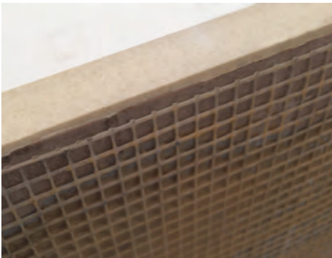
Backing with double fiberglass mesh.
