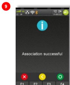
The terminal will automatically connect while sat on the cradle and will connect via ethernet while on the cradle, or within range for Bluetooth terminals.
