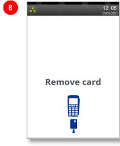
Tear off the receipt and remove the card, this will then initiate the printing of the customer receipt.
