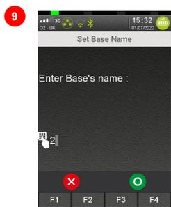
Enter the name you would like for the base using the number pad, then confirm this by pressing
