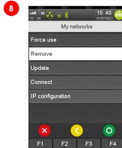
Select the “Remove” option using the touchscreen. This network will then be removed from the list of active networks.
