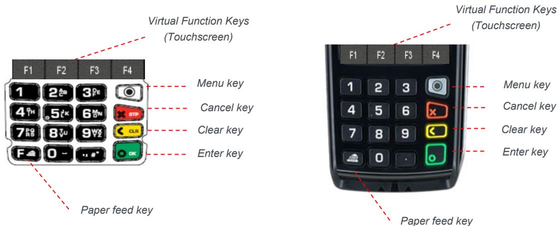
**Keypad Layout:** Depending on the model of your terminal it may come with one of the two above keypad layouts.
