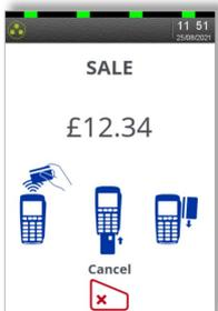
The contactless read is successful when all four status lights at the top of the screen are lit, and the confirmation tone is heard.
