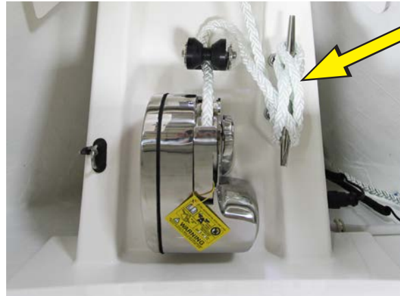
Windlass and anchor rode cleat (typical)
