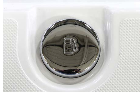
Gasoline fuel fill
