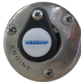
Engine flushing system hose connection
