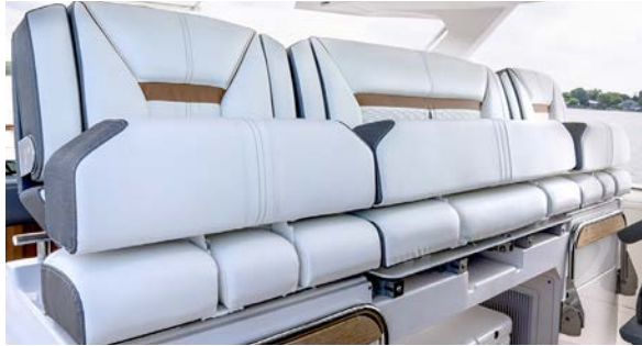
Helm seats with flip-up bolsters
