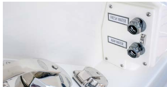
Optional fresh and raw washdown inlets in the aft starboard shorepower locker
