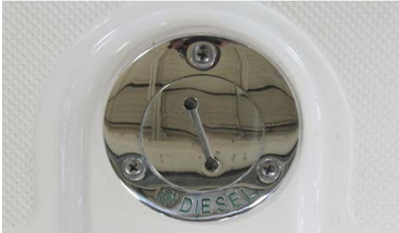
Diesel fuel fill
