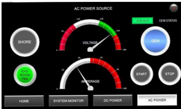
SHORE and GEN power buttons on the AC Power screen of the power-up panel
