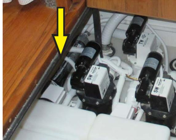
*Waste tank vent air filter indicated by arrow*
