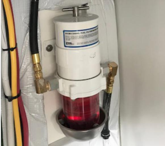
*Fuel water separating filter (typical)*
