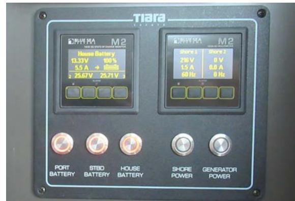
*Power Control Panel with AC voltage monitor.*
