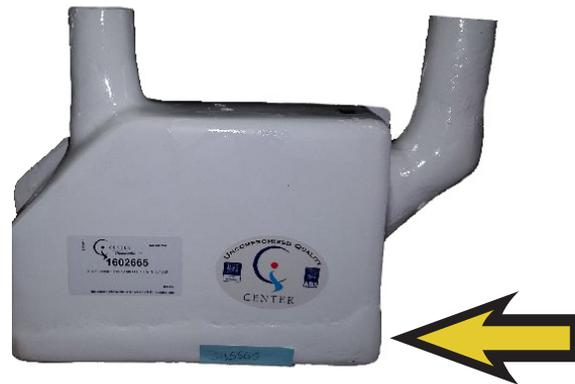
*Generator muffler drain plug*
