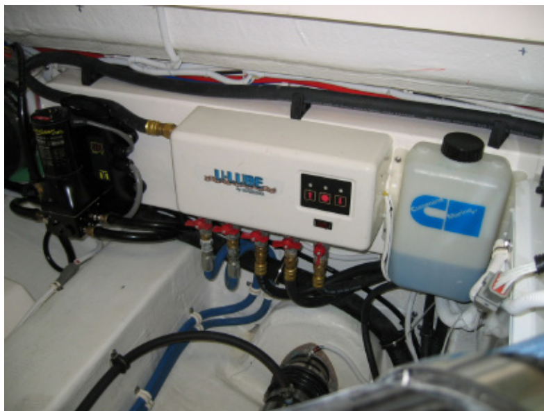
Figure 3-4: Aft of the starboard engine. From left to right: power assist steering pump, oil changer, and the starboard engine coolant recovery tank.
