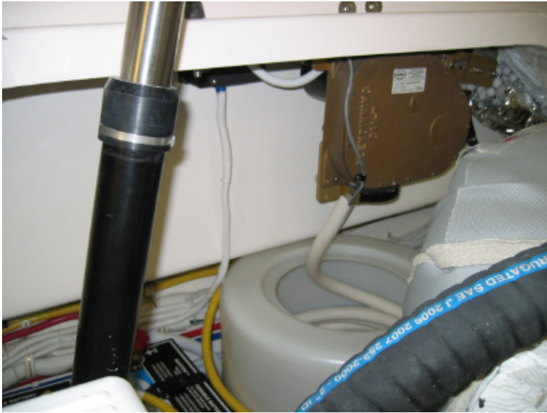
Figure 3-5: Storage bucket for the aft 50A, 240V shore power cable, outboard on starboard.
