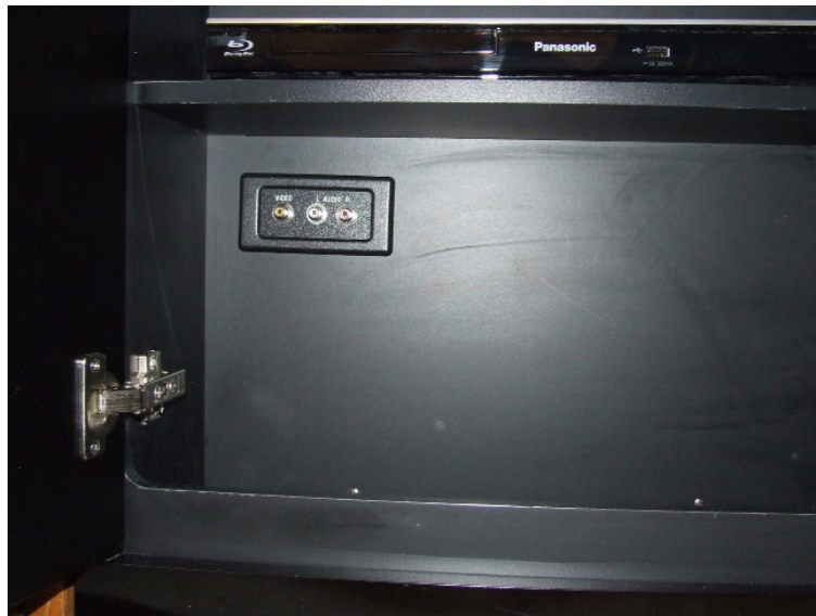
Figure 2-8: Audio video inputs located in the cabinet below the TV.
