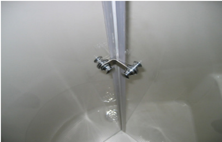
Figure 2-6: The bifold shower doors shown in the closed underway position. The lock clamps down on the left side handle. To use the doors for showering swing the lock open, open the right side door out and forward, then the left, meet the doors together and they will magnetically bond, as shown in Figure 2-7.
