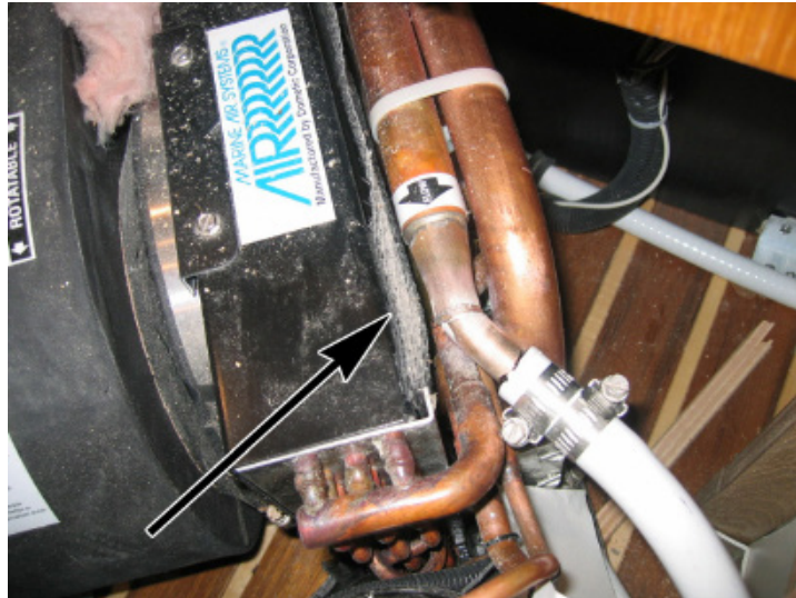
Figure 7-10: The A/C unit below the aft inboard dinette seat. The arrow points to the mesh filter.
