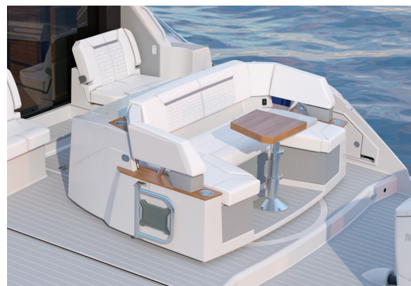
The rotating U-lounge rotated 180° to position the seat facing aft
