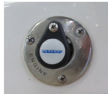
Engine freshwater flush hose connection (in the shorepower cabinet)
