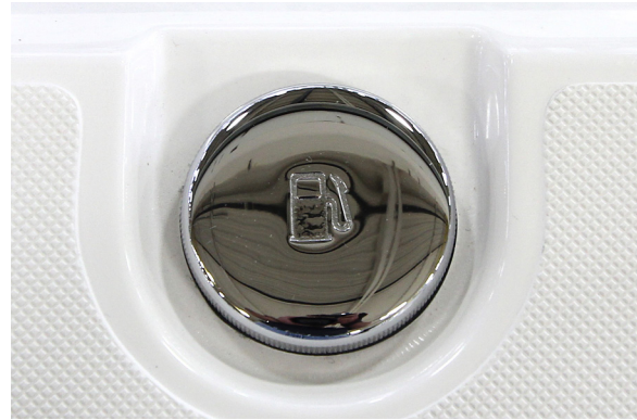
Gasoline fuel fill
