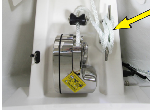
Windlass and anchor rode cleat (typical)
