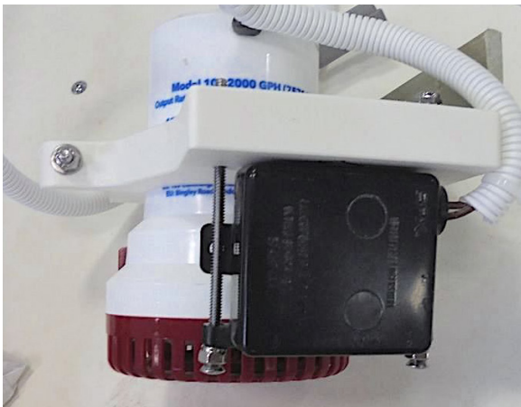
Typical bilge pump and float switch (right)
