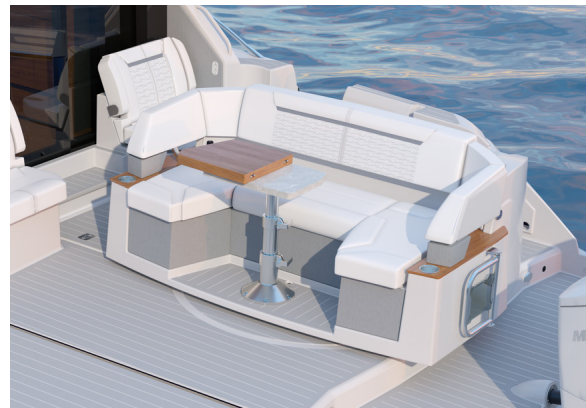
Use the SEAT AFT button to rotate the rotating U-lounge counterclockwise
