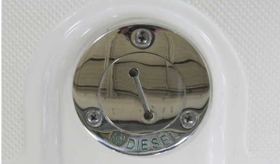
Diesel fuel fill
