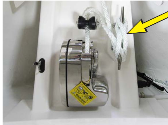
Windlass and anchor rode cleat (typical)
