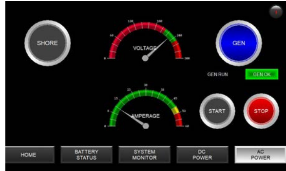
AC Power screen of the power-up panel, indicating that the generator is running.
