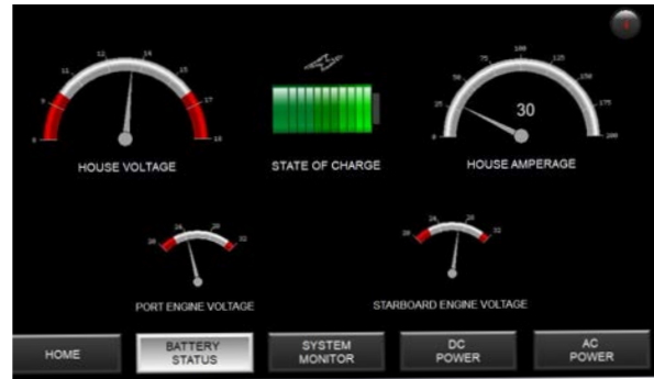
Battery Status screen
