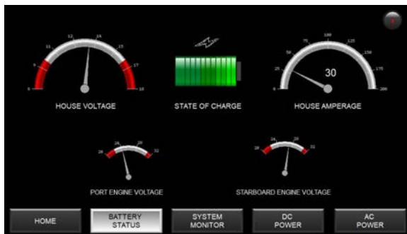
Battery Status screen, power-up panel
