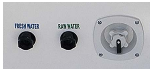
Fresh and raw washdown inlets are installed in the water connection locker under the aft transom port step and in the upper anchor locker
