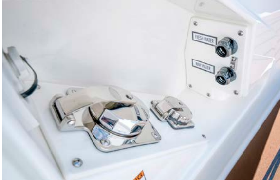
Shorepower and water connection cabinet
