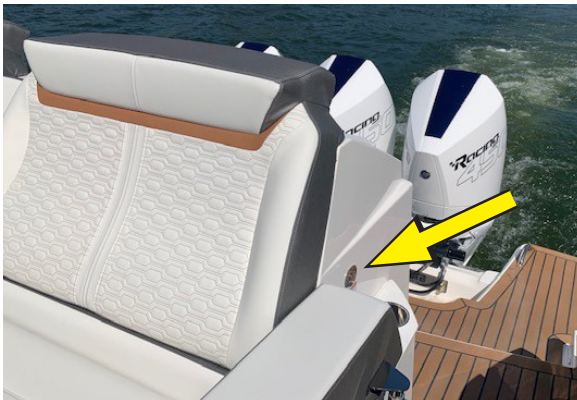
1. Disengage the latch found on aft lounge’s port side (when forward facing)
