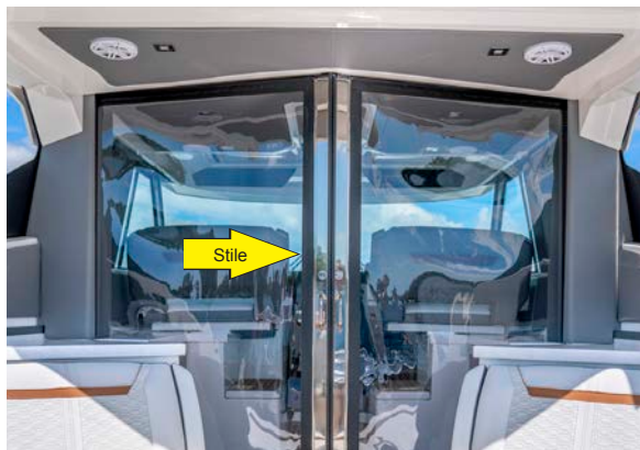
Retractable cockpit enclosure in latched position
