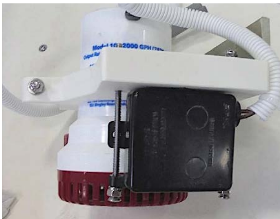
Typical bilge pump and float switch (right)
