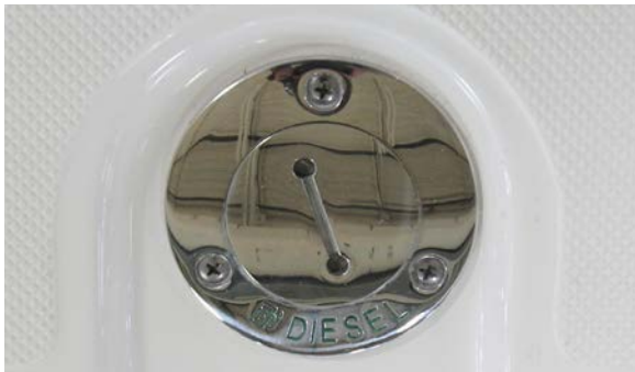
Diesel fuel fill
