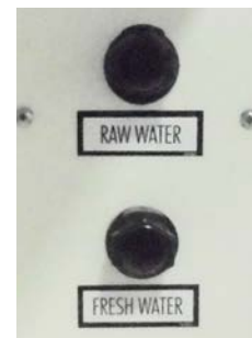
Optional fresh and raw washdown inlets, in the starboard foredeck fender storage area
