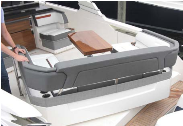
3. Rotate the cockpit to starboard
