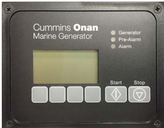
Remote generator control panel (typical)
