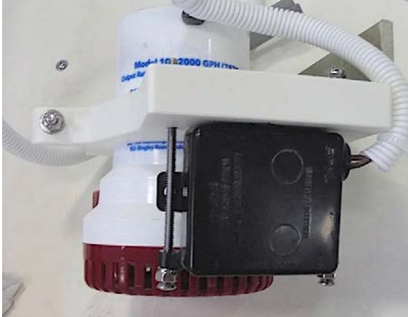
Typical bilge pump and float switch (right)
