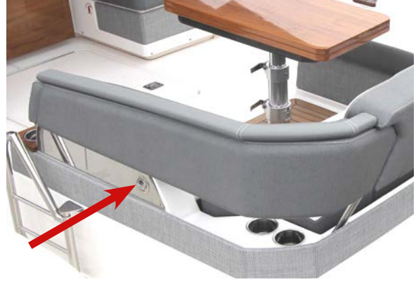
2. Disengage the latch found on U-lounge's port side (when forward facing)
