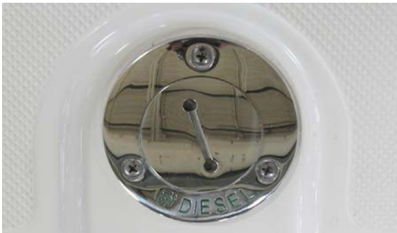
Diesel fuel fill
