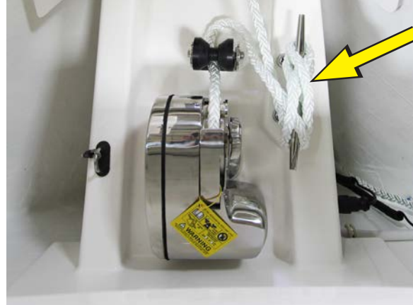
Windlass and anchor rode cleat (typical)
