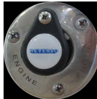
Engine flushing system hose connection
