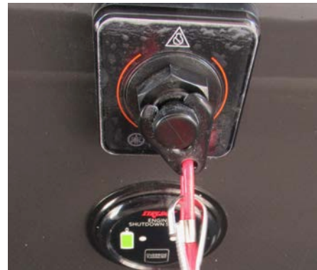
Engine stop switch and lanyard (typical)
