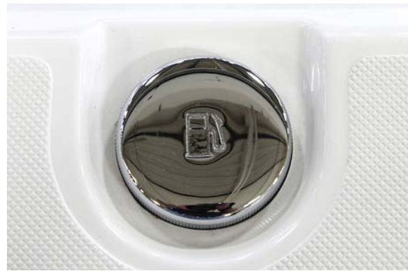
Gasoline fuel fill
