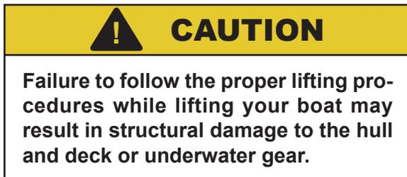
Severe gelcoat cracking or more serious hull damage can occur during hauling and launching if pressure is created on the gunwales (sheer) by the slings. Use flat, wide slings and spreaders long enough to keep pressure from the gunwales. DO NOT allow your boat to be hauled when the spreaders on the lift are not wide enough to take the pressure off the gunwales.
