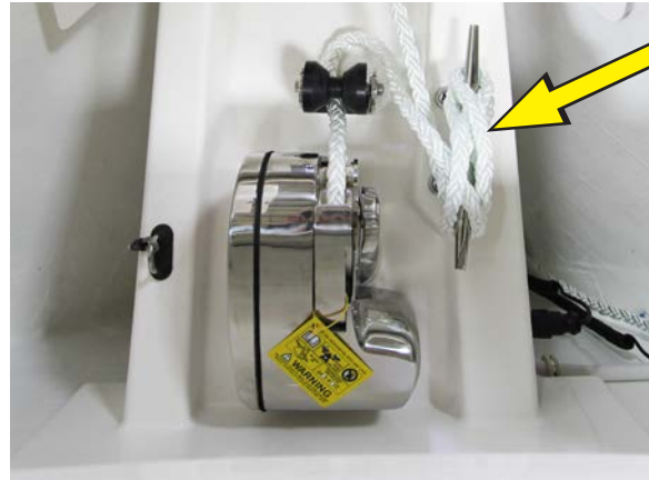
Windlass and anchor rode cleat (typical)
