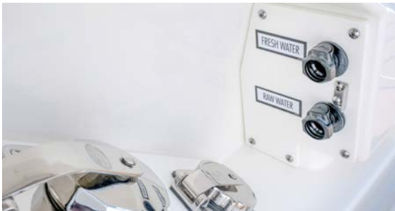
Fresh and (optional) raw washdown inlets in the aft starboard shorepower locker
