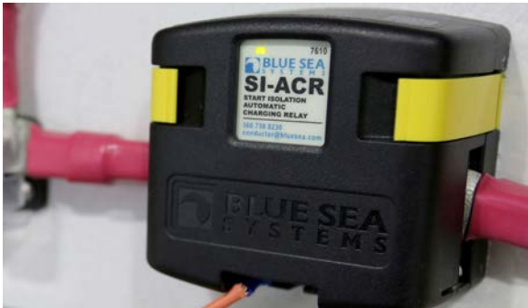
Automatic charging relay box (typical)
