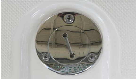
Diesel fuel fill
