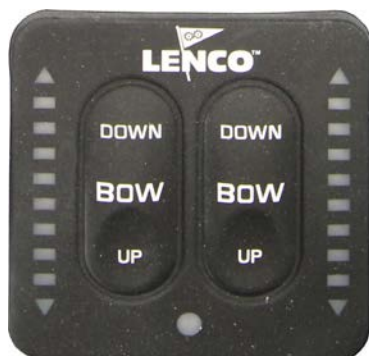
Trim tab switches
