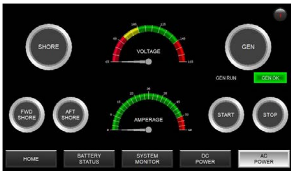
SHORE and GEN power buttons on the AC Power screen
