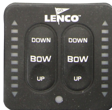
Trim tab switches
