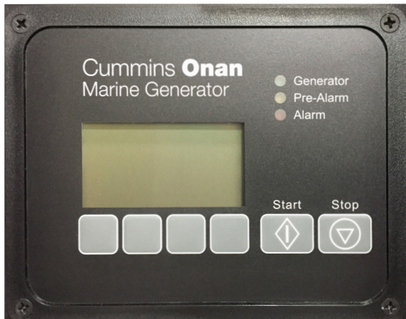
Remote generator control panel (typical)
