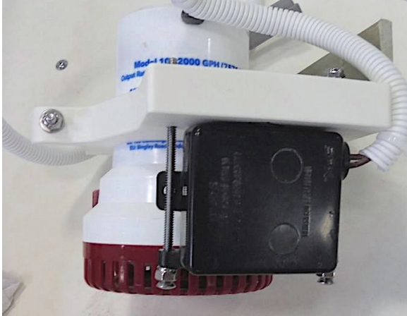
Typical bilge pump and float switch (right)
