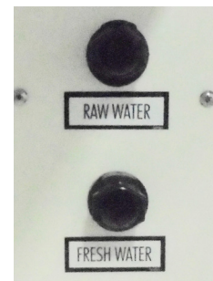
Optional fresh and raw washdown inlets, in the starboard foredeck fender storage area
