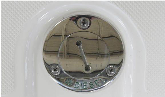
Diesel fuel fill
