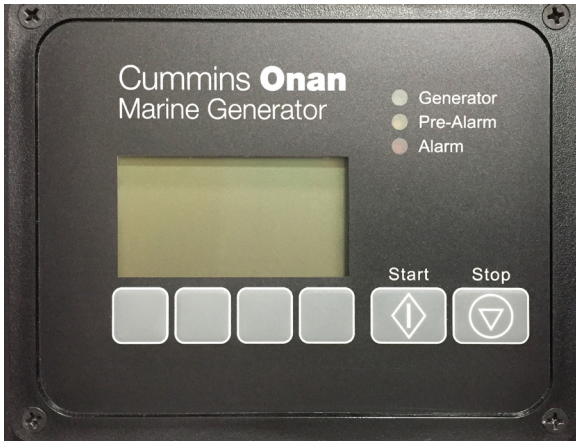
Remote generator control panel, in lower port companionway cabinet
