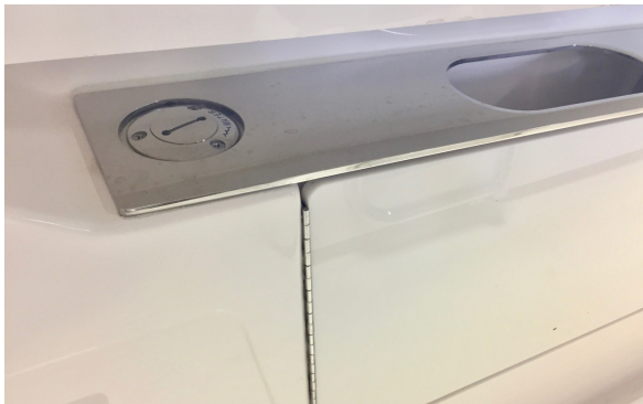
Water fill plate, aft cockpit under the starboard gunwale
