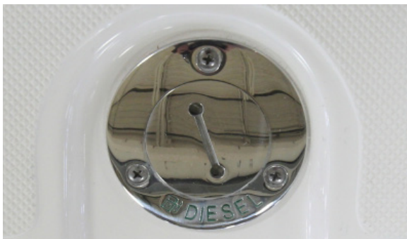
Diesel fuel fill
