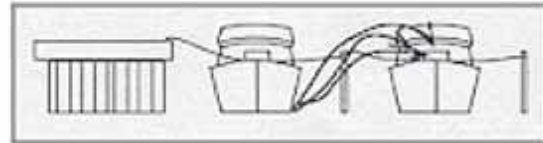
NEARBY BOAT GENERATOR EXHAUST
