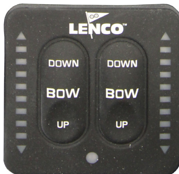
Trim tab switches
