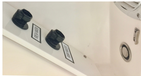
Fresh water and raw water washdown inlets in the water connection locker (optional)
