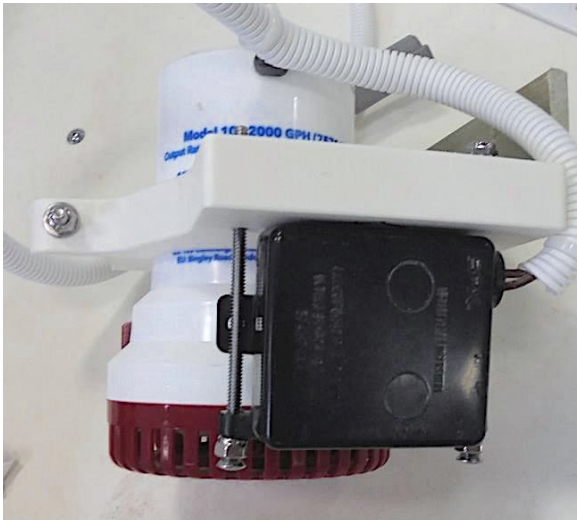
Typical bilge pump and float switch (right)
