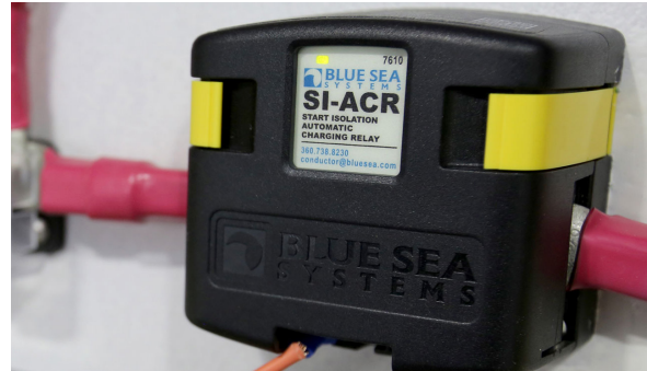
Automatic charging relay box (typical)
