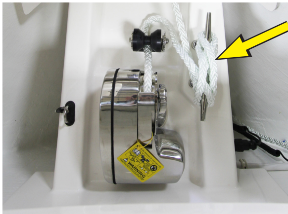
Windlass and anchor rode cleat (typical)
