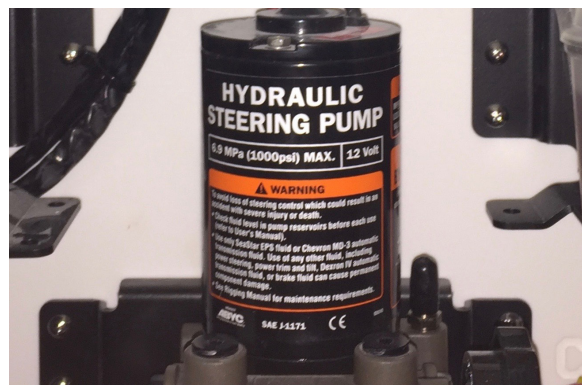
Steering pump (typical)
