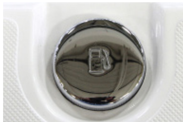
Gasoline fuel fill
