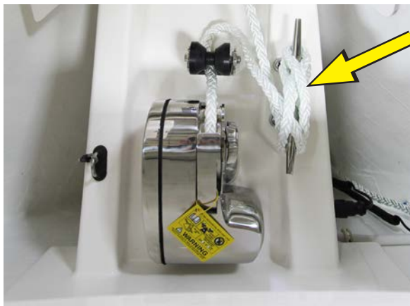
Windlass and anchor rode cleat (typical)
