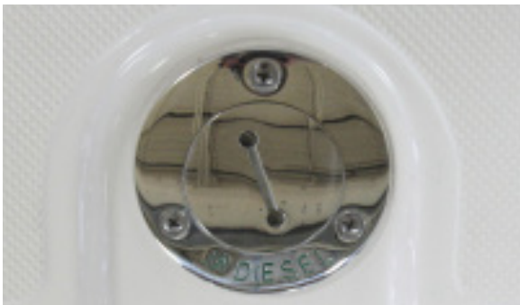
Diesel fuel fill
