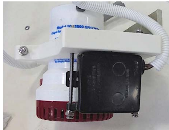
Typical bilge pump and float switch (right)
