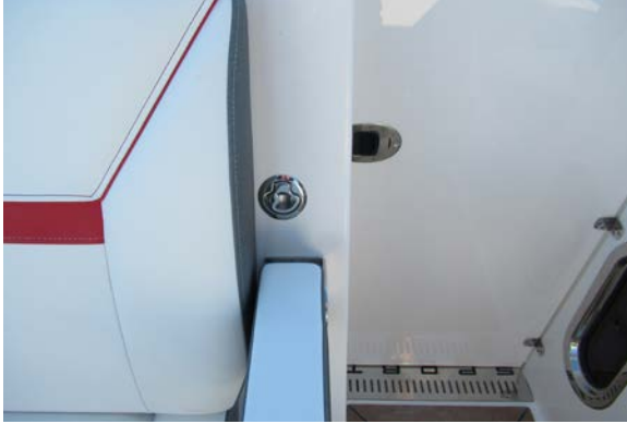
Toy storage compartment latch, above the starboard forward lounge seat armrest
