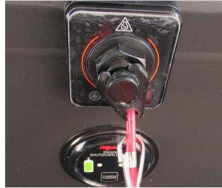
*Engine stop switch and lanyard (typical)*
