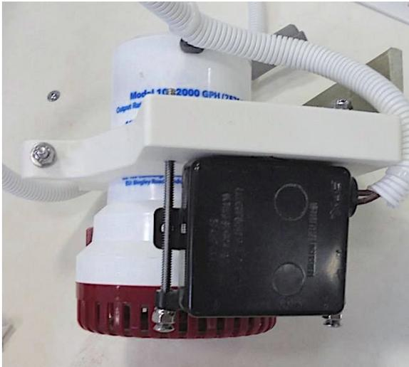
*Typical bilge pump and float switch (right)*
