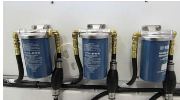
*Gasoline fuel water separating filters (typical)*
