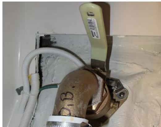
*Waste discharge seacock, under cabin floor hatch*
