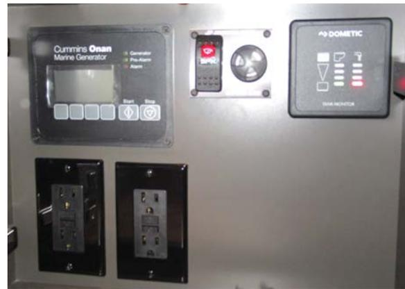
*Generator control; high water alarm; holding tank monitor; and outlets, in the port companionway lower cabinet*
