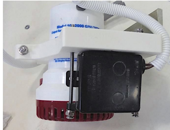
Typical bilge pump and float switch (right)
