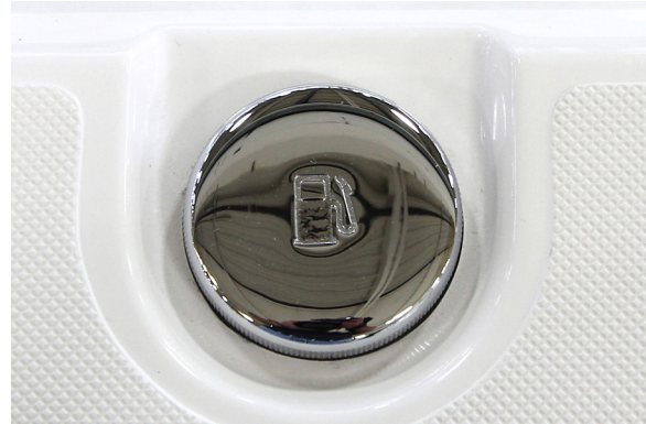
Gasoline fuel fill
