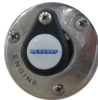
Engine flushing system hose connection
