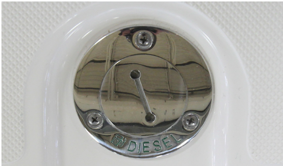
Diesel fuel fill
