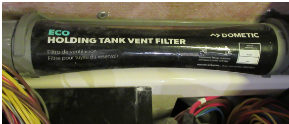
Tank vent filter, in the engine room on top of the holding tank
