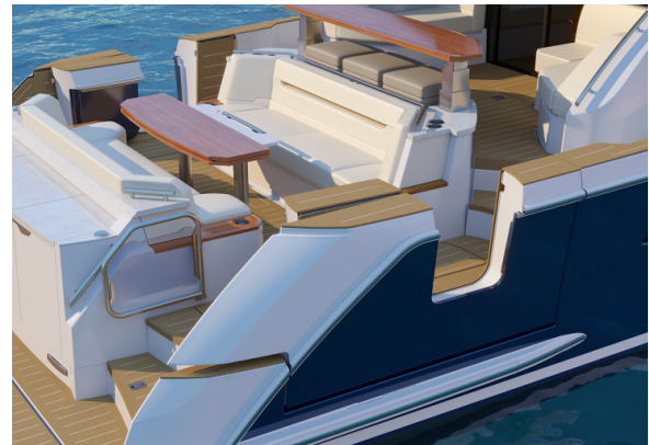
Hullside boarding doors, shown in the open position
