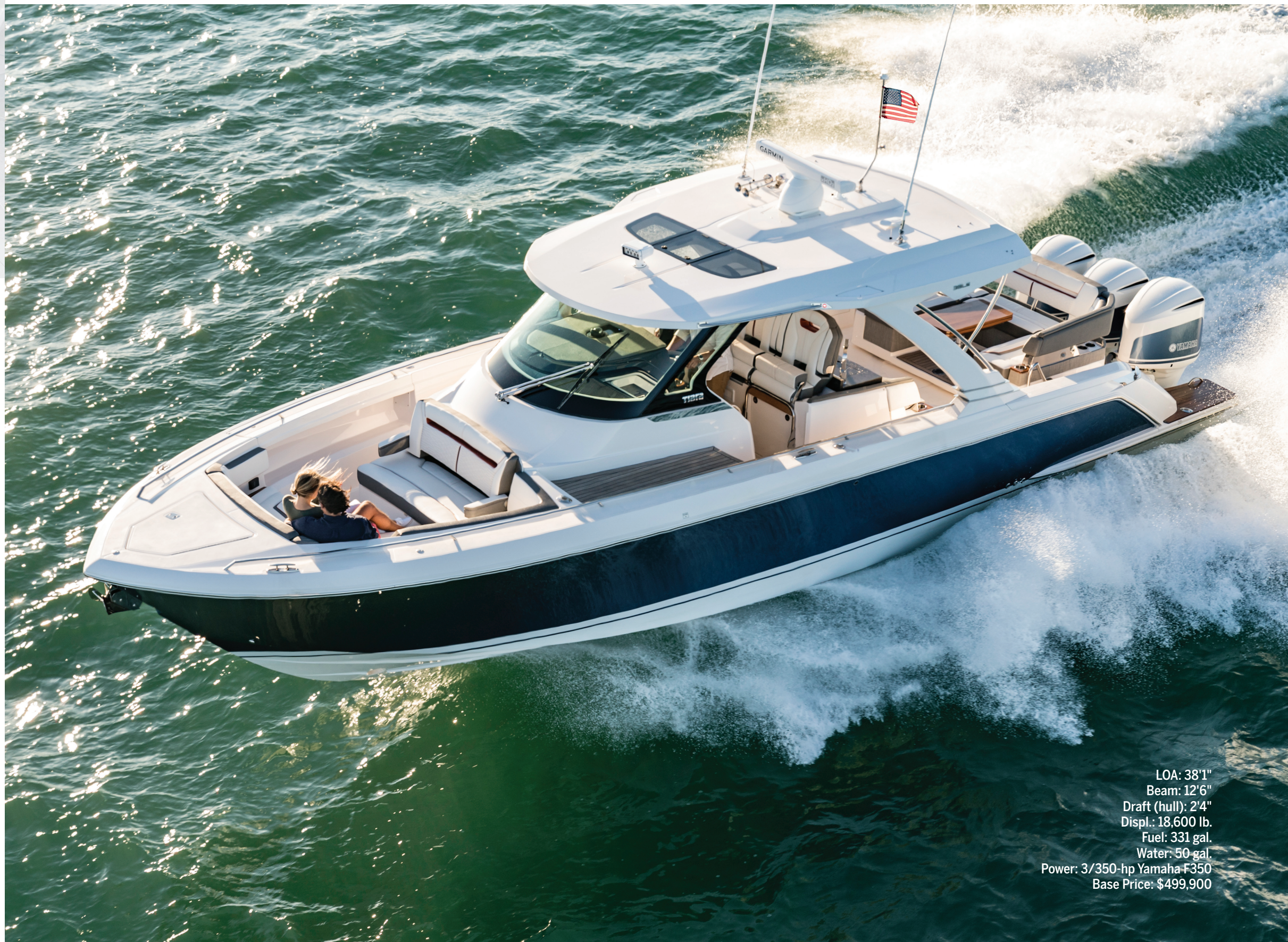
A trio of Yamaha F350s push the 38 LS to 49 knots at wide-open throttle.
