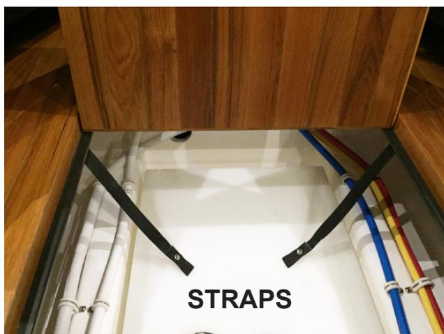
*Figure 2-3: Hatch straps*
