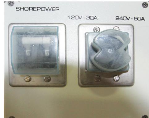
*Figure 4-10: Shore power breaker & selector switch*
