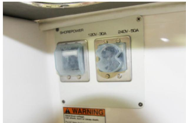
Figure 1-7: Power selection and breaker
