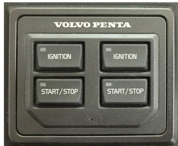
Figure 5-7: Volvo® e-Key control panel
