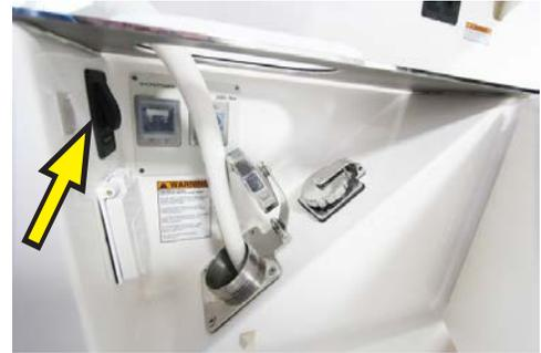
*Figure 5-2: Aft port shore power locker and cable master switch*
