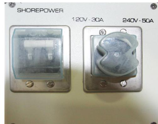
*Figure 5-1: Shore power breaker and selector switch*
