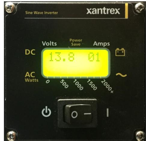
*Figure 4-11: Inverter control panel*
