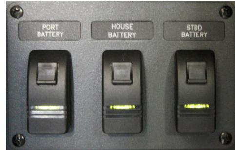
Figure 4-4: Battery Switch Panel
