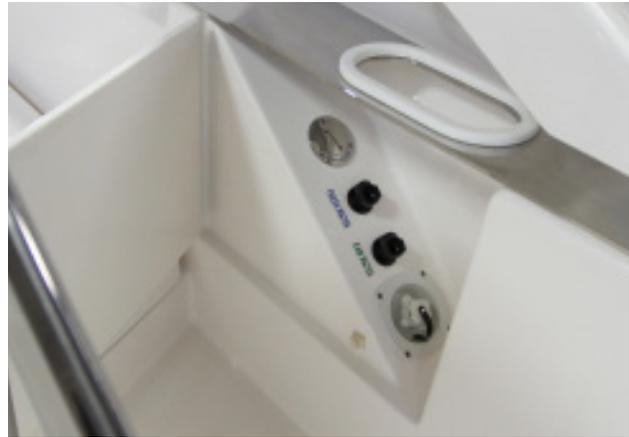
*Figure 1-8: Water connection locker*
