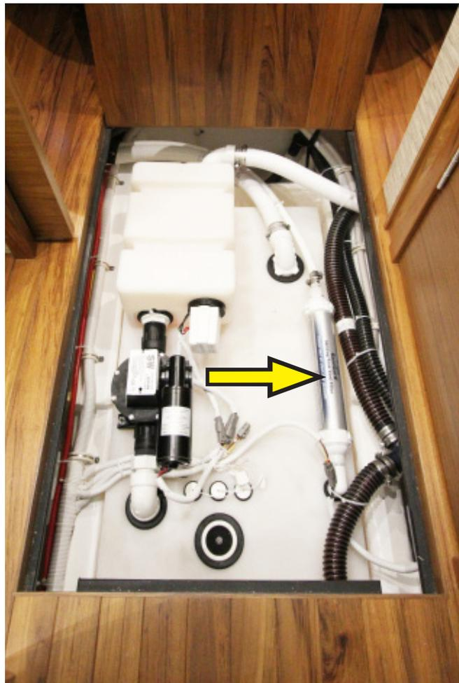
*Figure 7-4: Top of the waste tank (located under the atrium floor hatch). The tank vent air filter is indicated by the arrow.*
