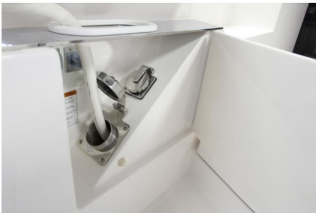
Figure 1-6: Aft shore power locker
