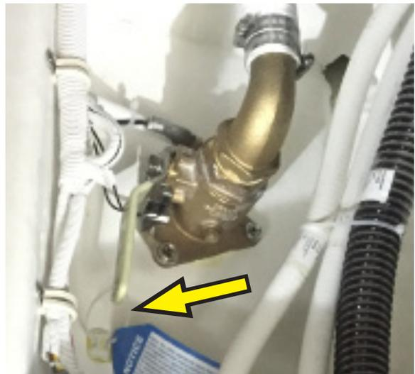
*Figure 7-6: Seacock in closed position and secured with cable tie*
