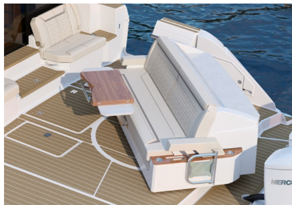
Use the SEAT AFT button to rotate the All-Sport counterclockwise
