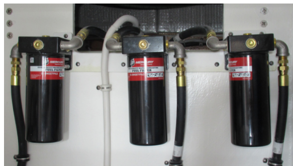
Gasoline fuel water separating filters (typical)
