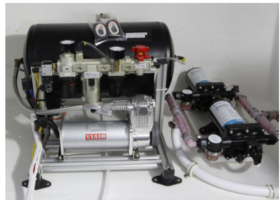
Figure 3-8: Air compressor and fresh water pumps
