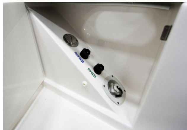
Figure 1-11: Water connection locker
