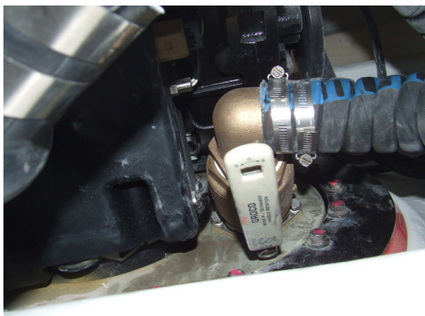
Figure 3-3: Zeus pod integral raw water seacock.
