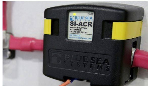
Automatic Charging Relay box (typical)
