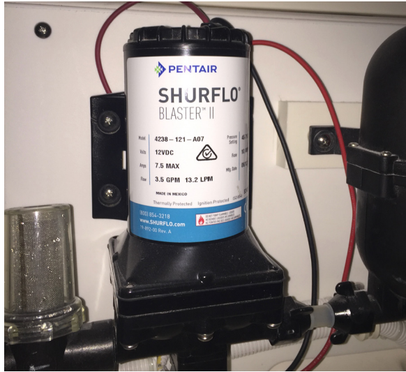
Raw water strainer (left) and pump (typical)
