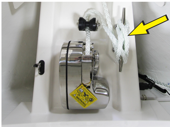
Windlass and anchor rode cleat (typical)
