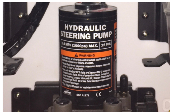
Steering pump (typical)
