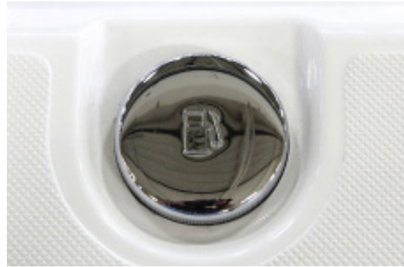
Gasoline fuel fill
