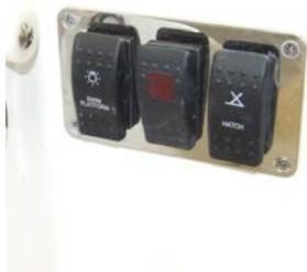
Figure 1-5: Switches on the port side of the transom buffet. From left to right: Optional hydraulic swim platform lift switch, optional underwater lights switch, transom hatch switch.
