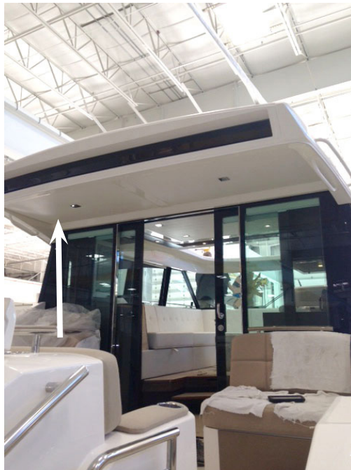
Figure 1-5: To check the sunshade fuse remove the port panel by pulling down. The fuse is located inside a gray control box.
