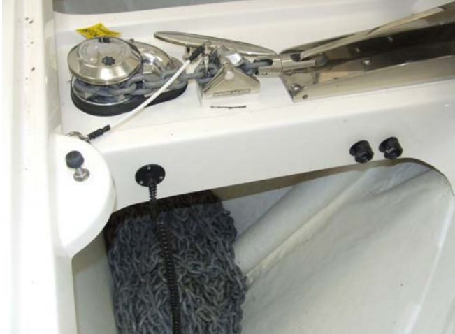
Figure 5-6: Windlass and ground tackle in the anchor locker.
