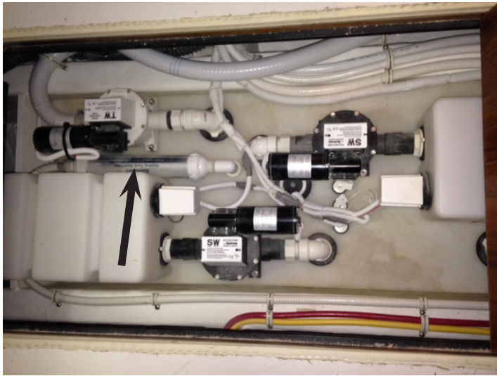
Figure 7-4: Top of the waste tank (top picture). A vent filter is located with the black arrow. Replace the vent filter annually.
