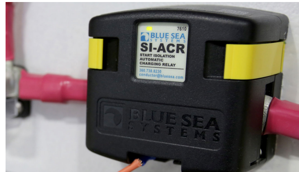
Automatic charging relay box (typical)
