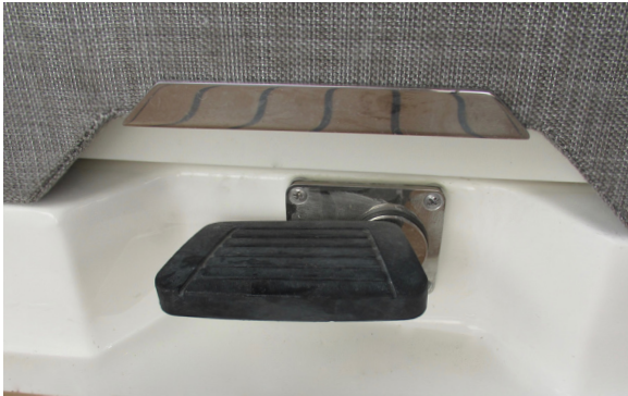
Aft lounge seat floor pedal for adjusting the backrest position
